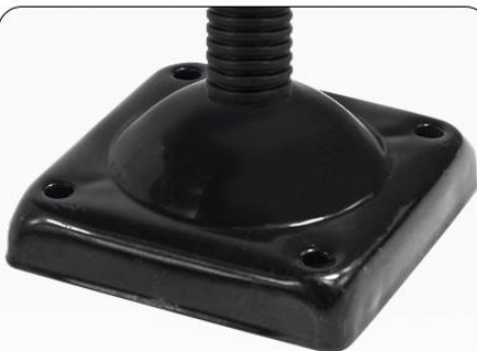
Large four-hole fixed lamp holder Mounting hole distance 60 mm. Hole diameter 7 mm.
